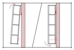
Hang the furniture unit on the top bar, allowing it to slide down into position. We recommend further securing the unit to the wall by driving 2 screws through the lower bracing bar.
