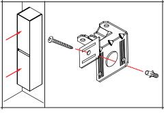
With the wall plugs in place, offer the unit to the wall and secure the screw through both mounting plates on each wall fixing.
