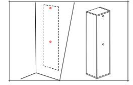
Make sure that there are no hidden pipes or cables in the wall. Drill 2 holes per mounting bar, using an 8mm drill bit to a depth of 55mm. The fixings supplied are for solid walls. For hollow or stud walls use specialist fixings.
